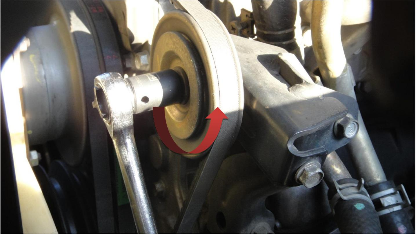
3. Use a 12mm socket. Turn the socket in increments of  $\frac{1}{2}$  turn to the right
