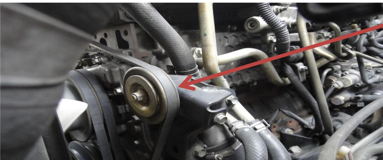
2. Used a 14mm socket to loosen nut **BUT DO NOT REMOVE**
