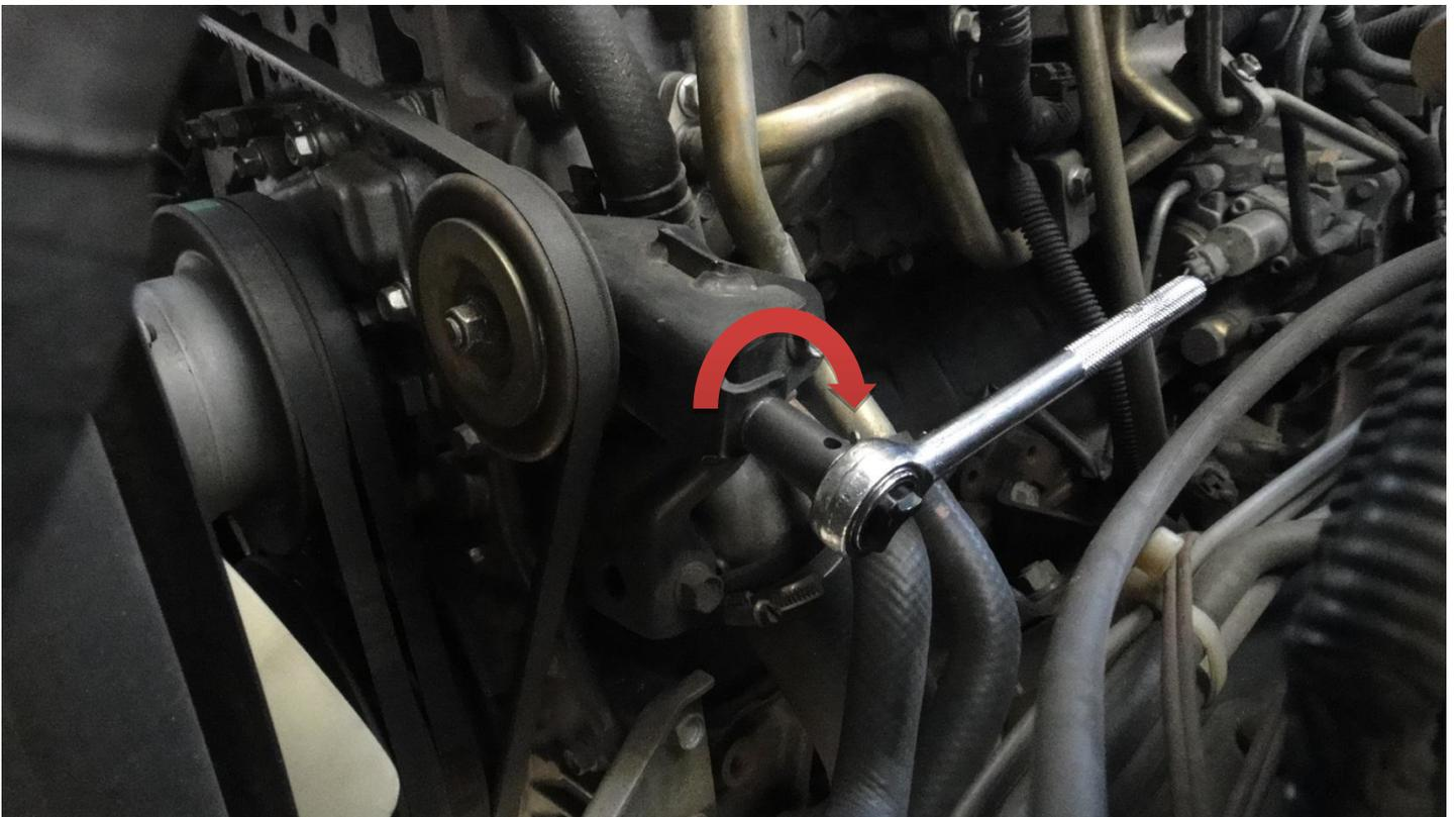
**Check the tension adjust if necessary but don't over do it**
